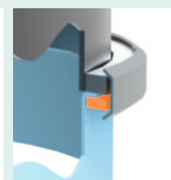
Clamping ring connection to the conventional flange system using an adapter
